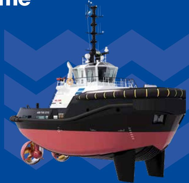
**Paramount for safe operations are good, predictable handling characteristics, along with extreme stability. This comes courtesy of the vessel's low profile, wide-beam combination with a patented Twin Fin skeg design.**
